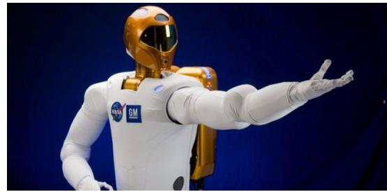
Known as Robonaut or R2, the robot was delivered to the space station in February and is being tested as an astronaut's helper.
